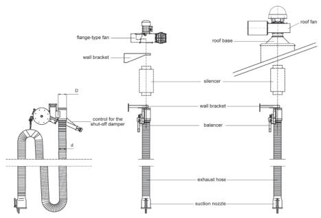
NOTE: Elements drawn in broken line are not belonging to the extractor set. On demand we deliver ventilation accessories (roof base, silencer etc.).
